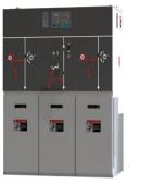
**RM Series** Extensible Moduler type Sf6 Gas Insulation and VI interruption Individual Circuit Breaker or Switch combination 12 ~ 27kV 630/1250A 20/25kA 125 BIL
